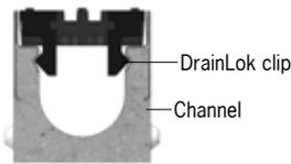
ACO DrainLok™ is a patented, boltless locking system that removes the need for bolts and bars and improves the hydraulic capacity of the channel. The DrainLok™ mechanism simply clips into the channel edge rail for rapid installation. ACO DrainLok™ grates are fitted with an anti-shunt mechanism that restricts unwanted grate movement when installed, improving durability and longevity of the system.
